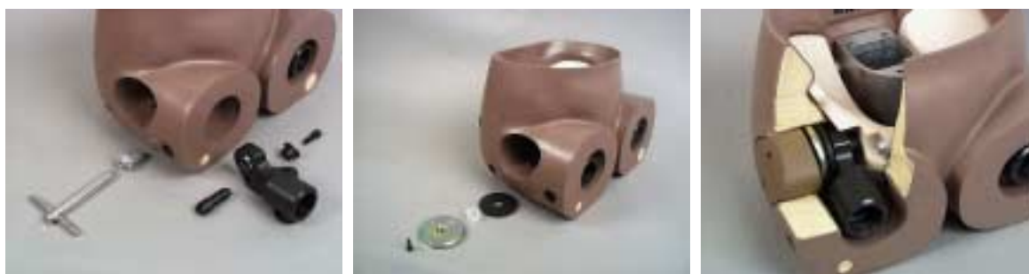
Figure 7: ES-2 pelvis assembly Left : New upper femur bracket with attachment pin Middle : H-point back plate with tube stop and H-point back plate buffer for abduction Right : Pelvis assembly (flesh foam partly cut away)
