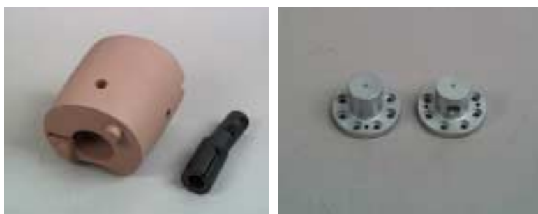
Figure 8: ES-2 leg parts modified Left : Upper leg thigh flesh foam part (left) and femur bone steel part (right) Right : Aluminium femur load cell end pieces (the dowel pin hole locations are not correct)
