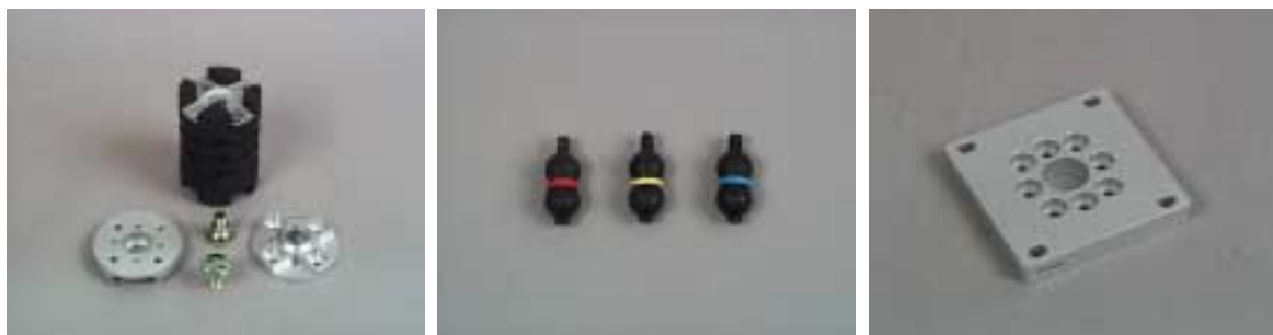
Figure 3: ES-2 prototype neck component Left : Central moulding, top and bottom interface plates and half spherical screws Middle : Buffers three harnesses Right : New neck to head form interface plate for certification
