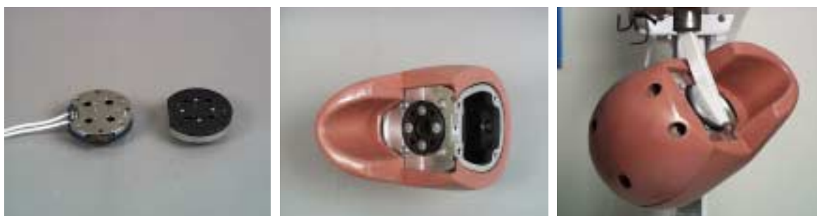
Figure 2: ES-2 Prototype head assembly Left : Upper neck load cell and its structural replacement Middle : Skull skin and structural replacement Right : Head assembly with head drop bracket in certification rig.
