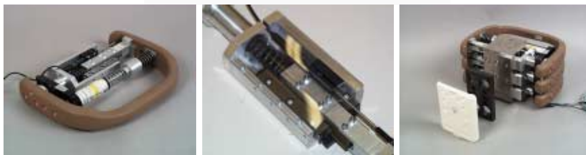
Figure 5: ES-2 Prototype thorax assembly Top : ES-2 rib unit with the newly designed needle bearing guide system Left : ES-2 rib unit assembly Middle : ES-2 needle bearing rib guide system with protection cover Right : ES-2 thorax assembly (ribs, spine box, replacement load cell and curved back plate)
