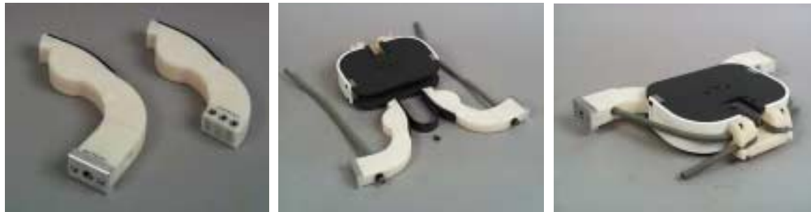
Figure 4: ES-2 Prototype shoulder assembly Left : Cam clavicle standard (left) and shortened for clavicle load cell application (right) Middle : Shoulder assembly (exploded) Right : Shoulder assembly (from aft side) note the new elastic cord holder
