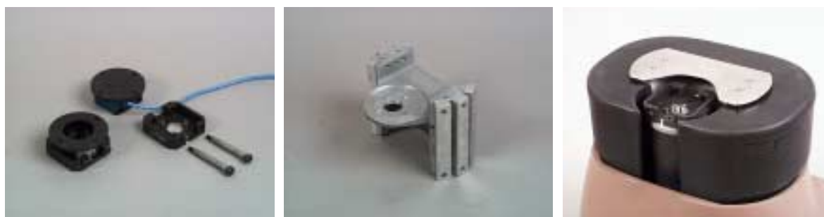
Figure 6: ES-2 Prototype abdomen assembly. Top : T12 load cell with base adapter and accelerometer mountings (Denton model 4284). Left : T12 load cell, base adapter and shoulder bolts (apart) and structural replacement and base adapter (assembled). Middle : Abdomen drum (with four hole in lug) Right : Abdomen assembly with base adapter on top.
