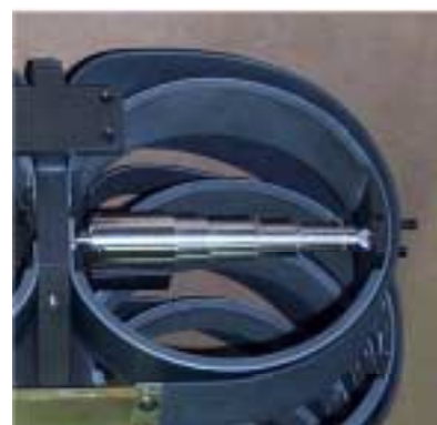
Figure 7: Outer and inner shoulder rib with IR-TRACC displacement transducer
