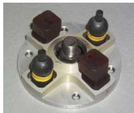
Figure 5: Detail of WorldSID neck buffers
