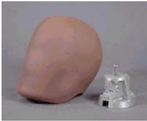
Figure 2: WorldSID head and instrumentation core Figure 3: Detail of head instrumentation core
