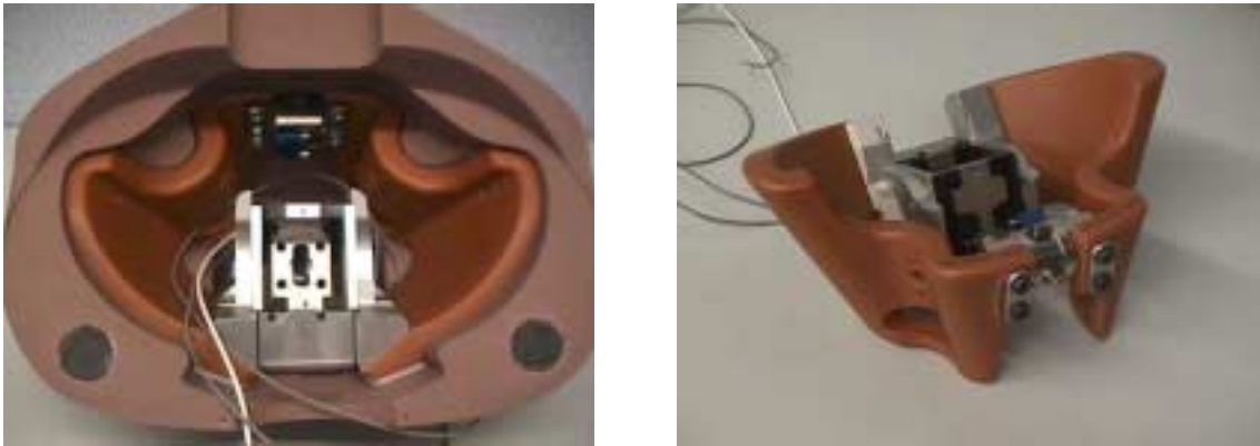
Figure 10: Pelvis assembly with and without flesh
