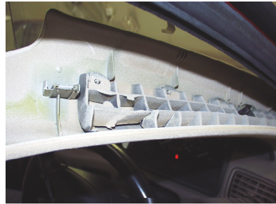
Figure 7. Roof rail padding of the Toyota Camry after the EC test.
