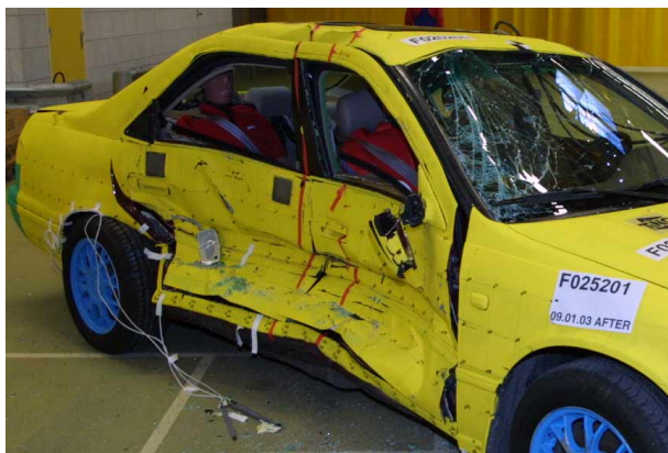
Figure 13 Camry after impact by the IIHS barrier face
