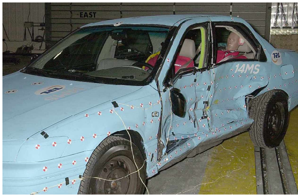
Figure 12 Camry after impact by the AE-MDB barrier face
