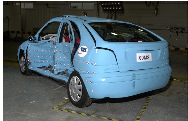
Figure 8 Megane after impact by the AE-MDB barrier face
