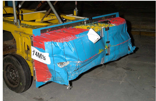
Figure 14 AE-MDB post impact deformation – Camry
