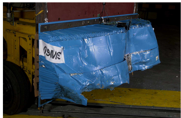
Figure 10 AE-MDB post impact deformation – Megane
