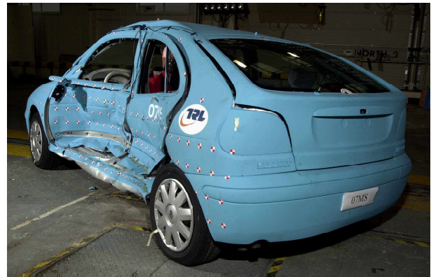
Figure 9 Megane after impact by the IIHS barrier face
