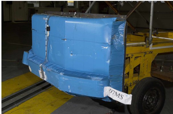
Figure 11 IIHS post impact deformation - Megane
