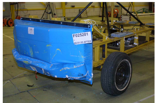
Figure 15 IIHS post impact deformation - Camry
