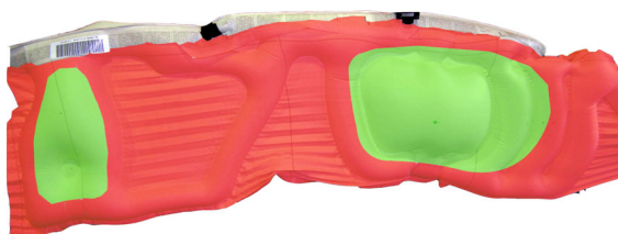
Figure 12: Marked protection level on airbag
