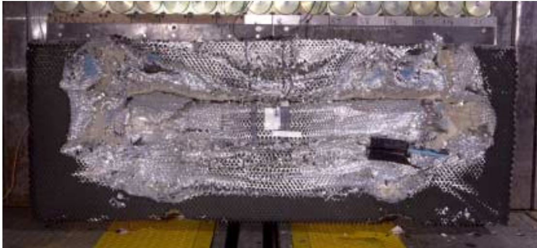
Figure 56: View of the resultant barrier deformation.
