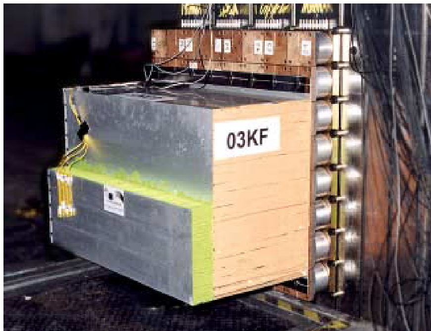
Figure 161: Offset deformable barrier (ODB) mounted onto high resolution load cell wall.
