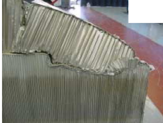
Figure 102: Barrier deformation showing the failure of the stiffer progressive layer prior to the softer front layer.
