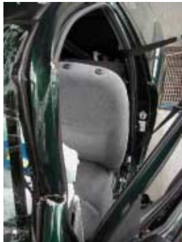
Figure 159: Toyota Yaris: driver seat rotation
