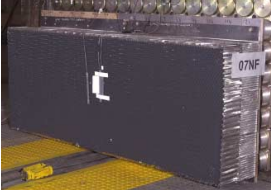
Figure 53: Full width test barrier mounted onto load cell wall.
