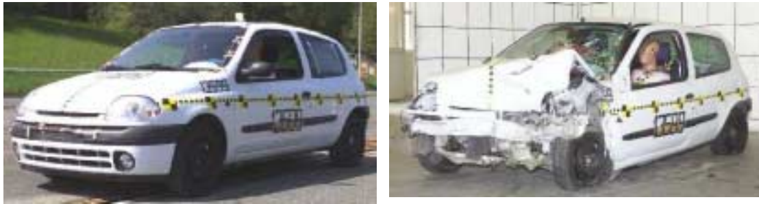
Figure 149: Renault Clio: pre and post test driver's angled view
