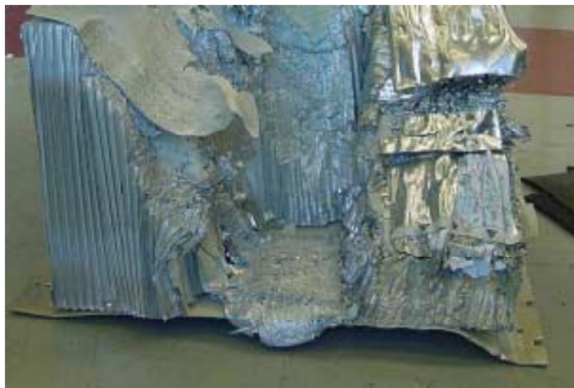
Figure 106: Progressive deformable barrier post impact showing bottoming out of barrier post impact.
