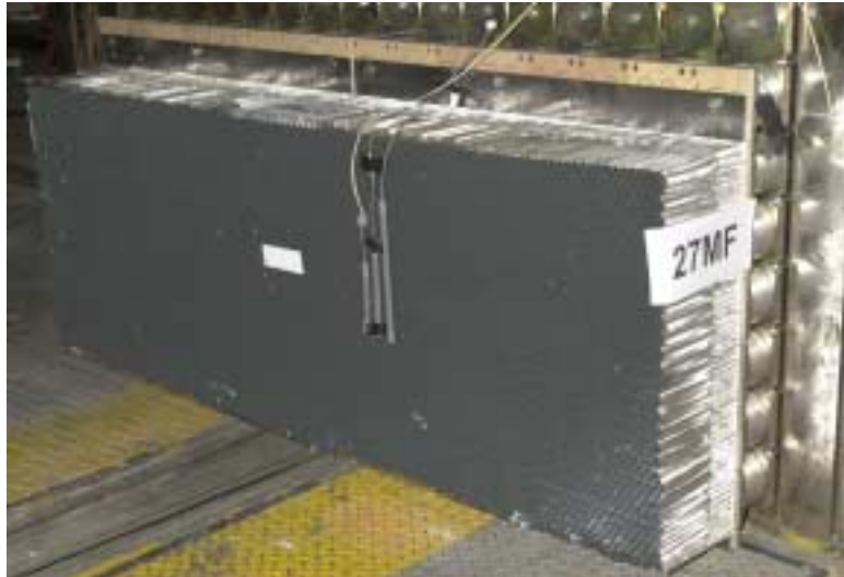
Figure 43: Development full width test barrier mounted onto load cell wall.
