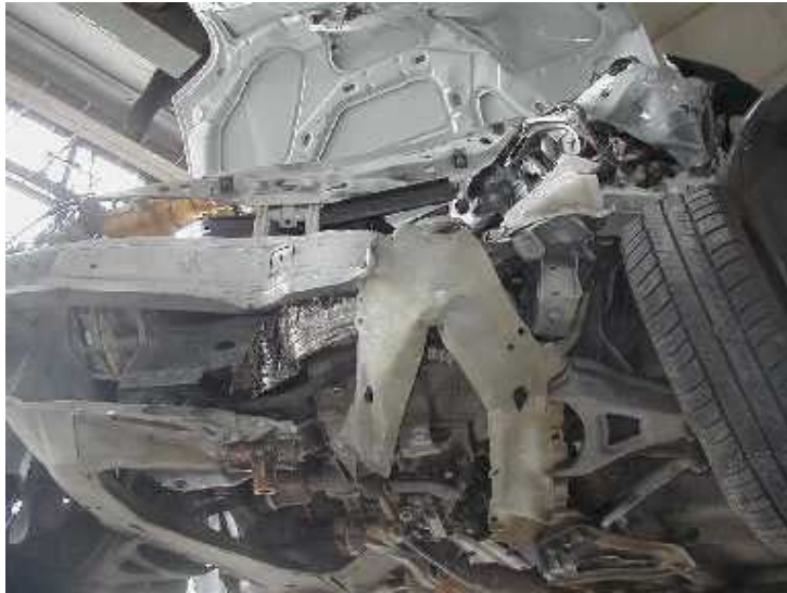
Figure 153: Renault Clio: sub-frame cut from Yaris wheel
