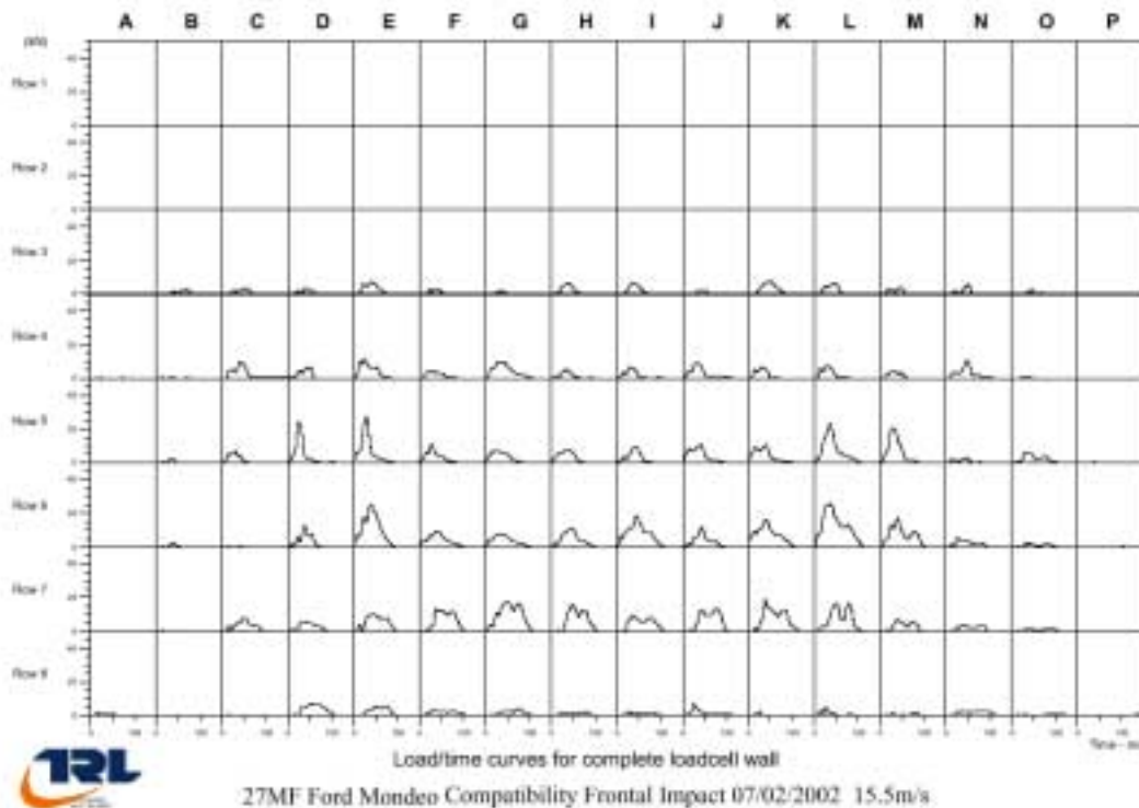
Figure 50: Load cell wall force time history showing the high loads applied by the lower rails and subframe crossbeam.
