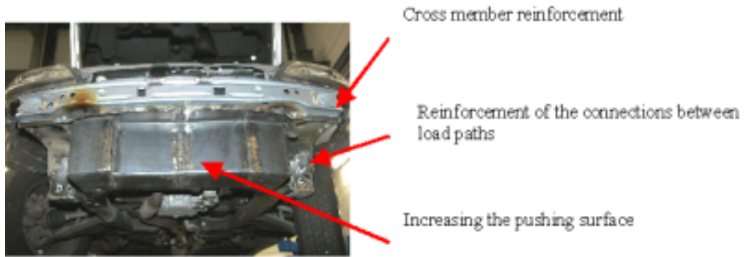
Figure 70: Modifications of the Opel Astra
