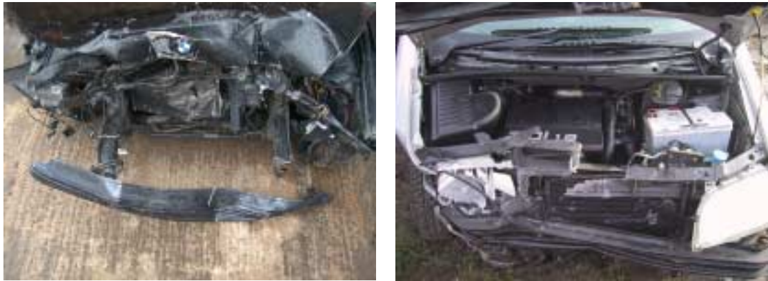
Figure 15: Comparison of damage to BMW and Sharan, showing lack of energy absorption in the frontal structures
