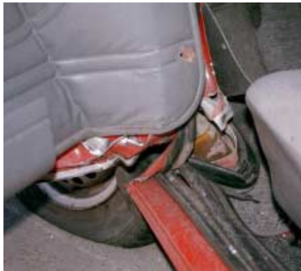
Figure 30: Deformation of the Passenger Compartment of the Corsa
