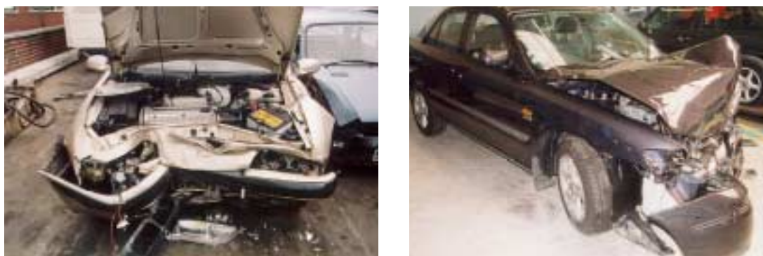
Figure 5: Comparison of the damage profiles of the Daewoo and Mazda, showing deformation of less stiff structure between longitudinals on the Daewoo
