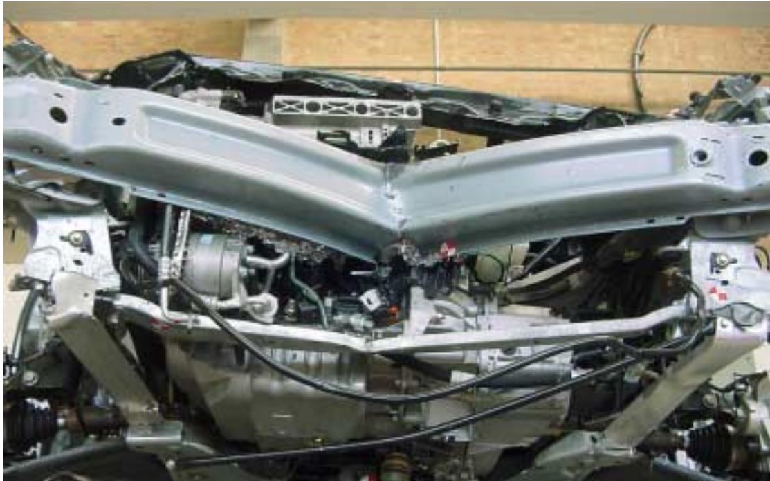
Figure 62: Centre of bumper beam and subframe crossbeam, showing bending failures.
