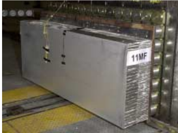
Figure 33: Development full width test barrier mounted onto load cell wall.
