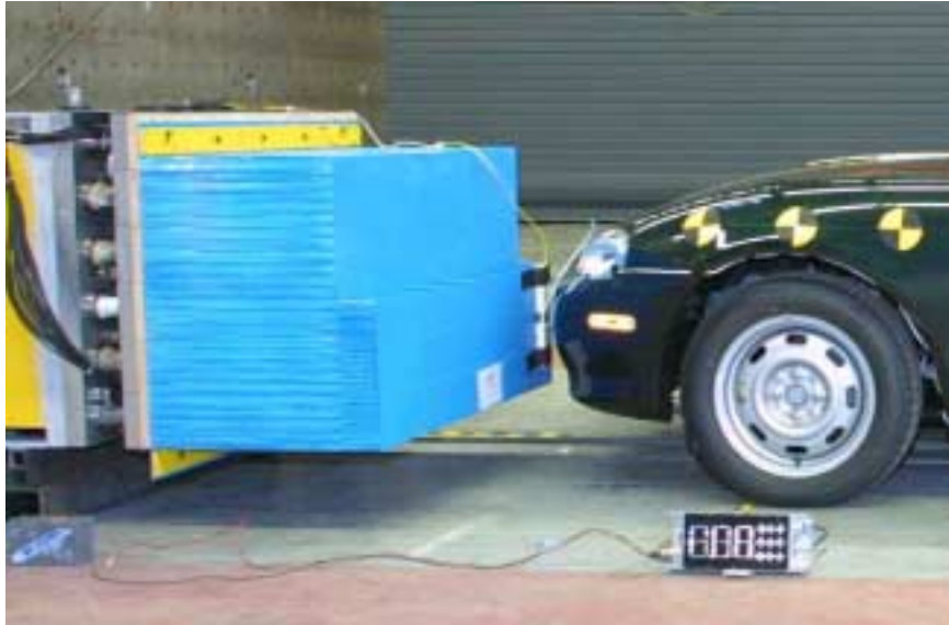
Figure 177: Euro NCAP Frontal Impact Barrier mounted to the Load Cell Wall
