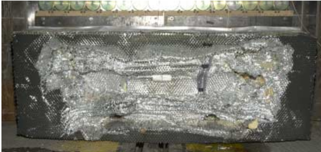
Figure 46: View of the resultant barrier deformation.
