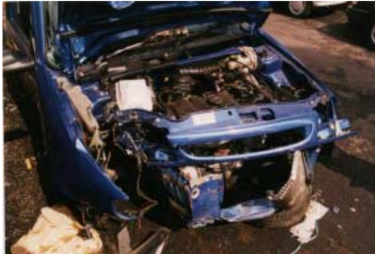
Figure 25: Citroen Saxo showing impact between upper and lower rails
