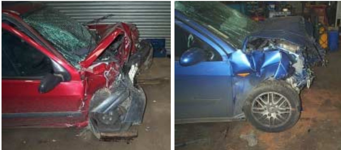
Figure 11: Comparison of the damage profiles of the Clio and Focus, showing that the Clio has been overridden
