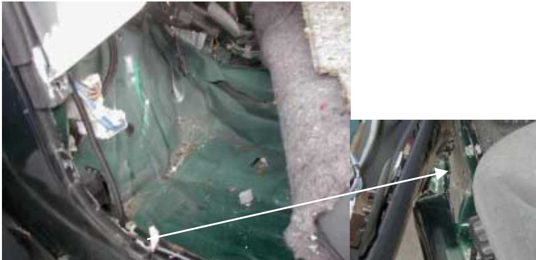
Figure 157: Toyota Yaris: Intrusions at low level of occupant compartment
