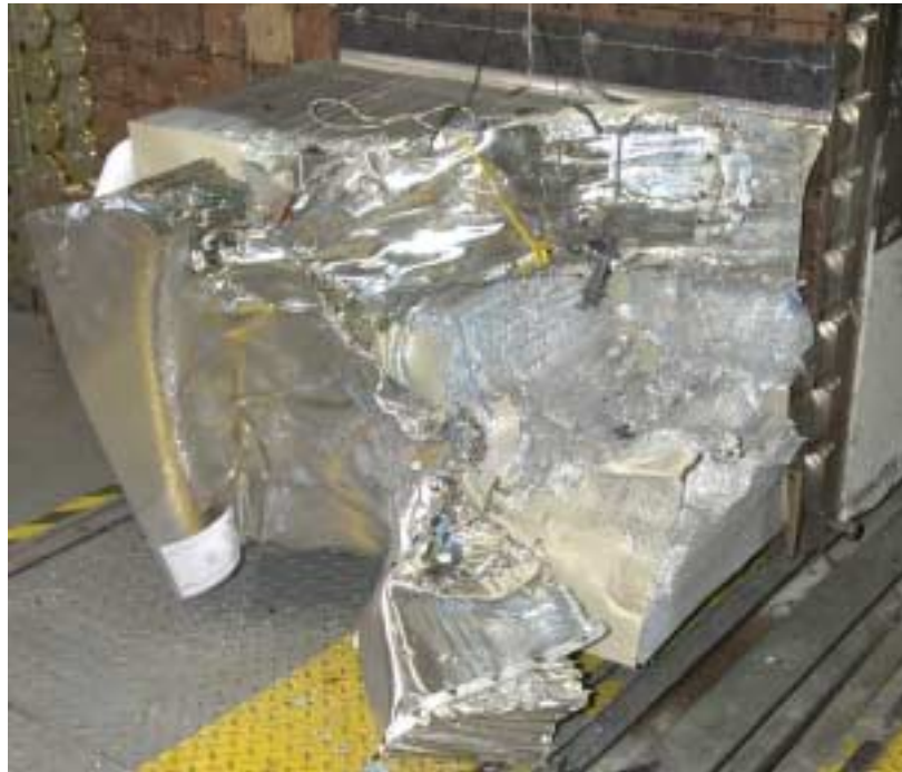
Figure 105: Progressive deformable barrier post impact showing bottoming out of barrier.
