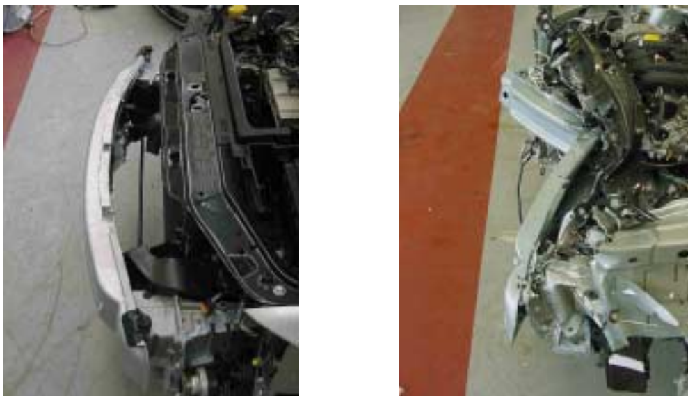
Figure 61: Comparison of bumper beam, pre and post-test, showing failure between lower rails.
