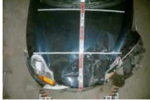
Figure 29: Front Deformation Porsche
