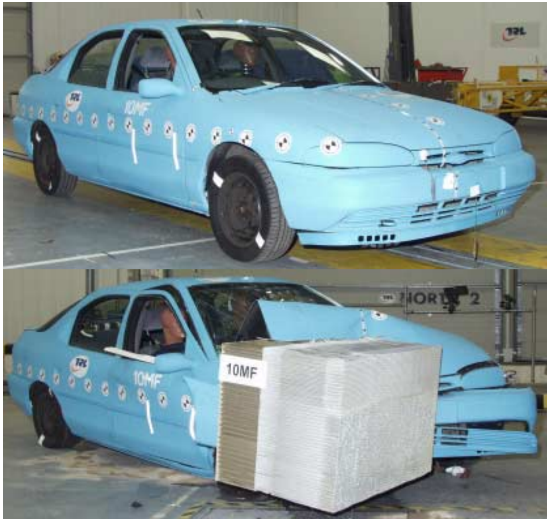
Figure 90: Vehicle pre and post test views showing the attachment of the barrier to the vehicle post impact.
