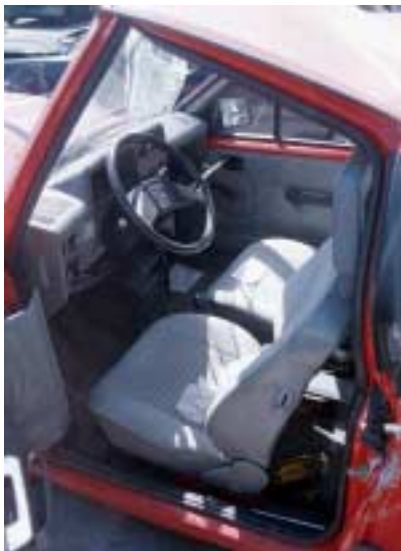
Figure 30: Deformation of the Passenger Compartment of the Corsa
