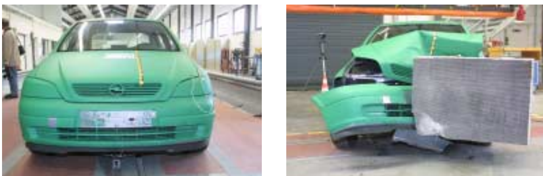
Figure 124: Vehicle pre and post Test Front View, Test 02CO14FO
