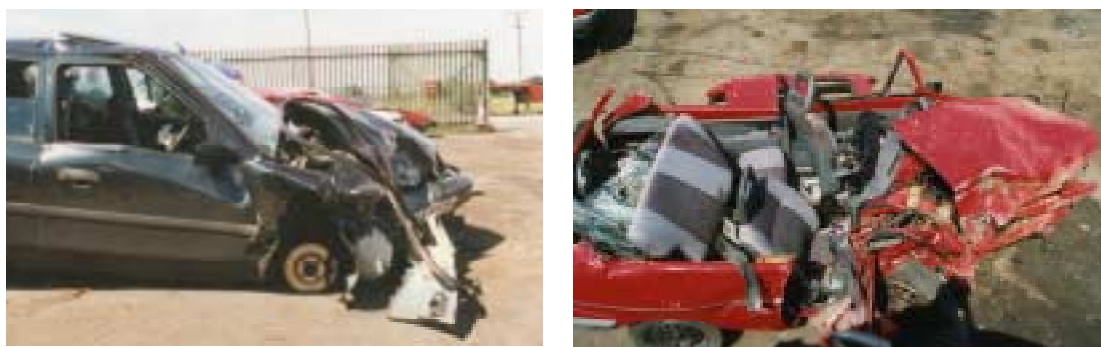
Figure 23: Comparison of vehicle damage for Mondeo and Fiesta, showing that the Fiesta has been overcrushed
