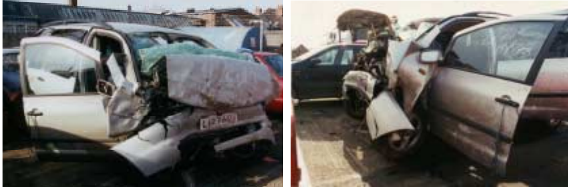
Figure 2: Seat Alhambra showing homogeneous deformation of frontal structure
