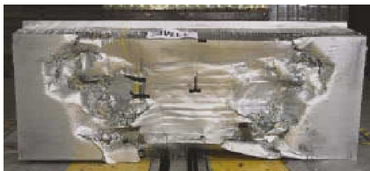
Figure 36: View of the resultant barrier deformation.
