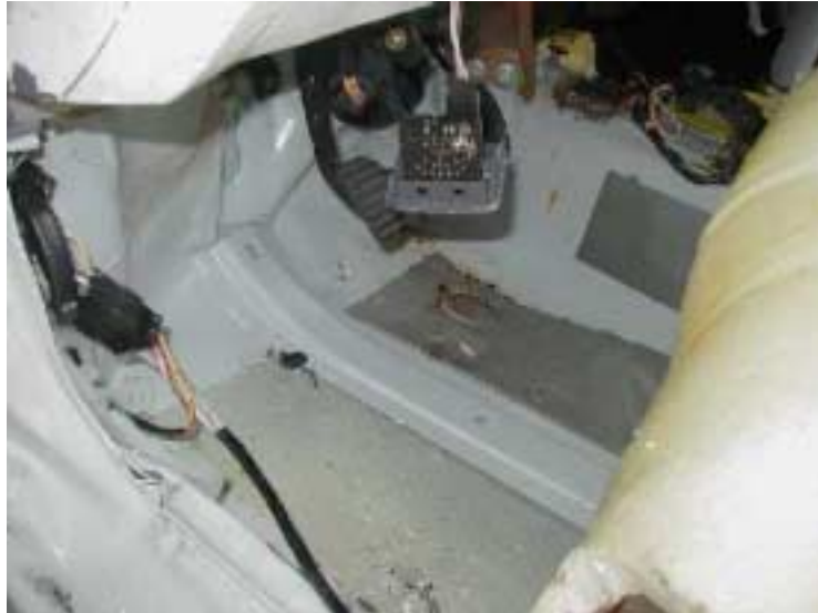
Figure 158: Renault Clio: Intrusions at low level of occupant compartment
