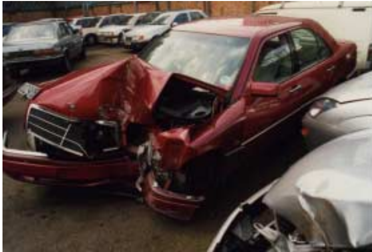
Figure 24: Mercedes C-180 showing narrow impact between longitudinals
