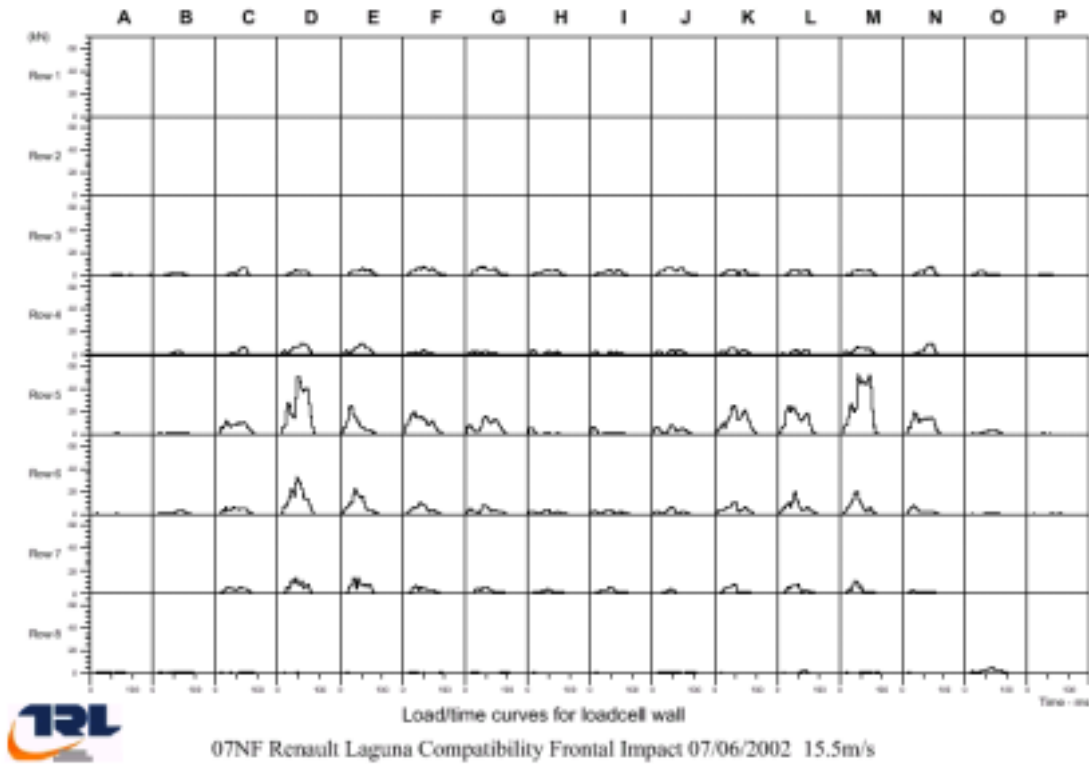
Figure 59: Load cell wall force time history showing the high loads applied by the lower rails.
