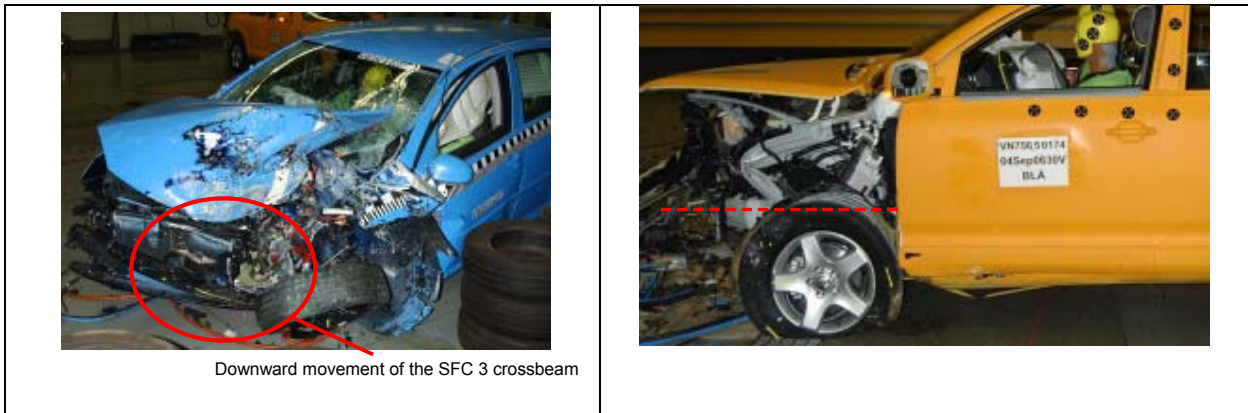
Figure 40: Deformation of the SFC 3 and SUV 2 showing the downward movement of the SFC 3 lower rail and the limited vertical movement of the SUV 2 lower rail
