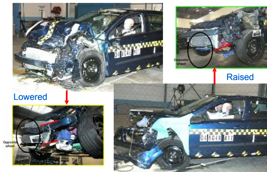
Figure 27: Car-to-car test with two load path level SFC 2, showing the contact of the impact side front wheel with the subframe crossbeam of the opposing car.
