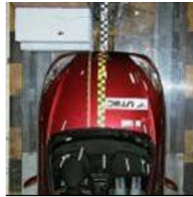
EEVC WG16 proposal: - Test Speed: 60 km/h - Overlap: 40 % - Barrier: current ODB
