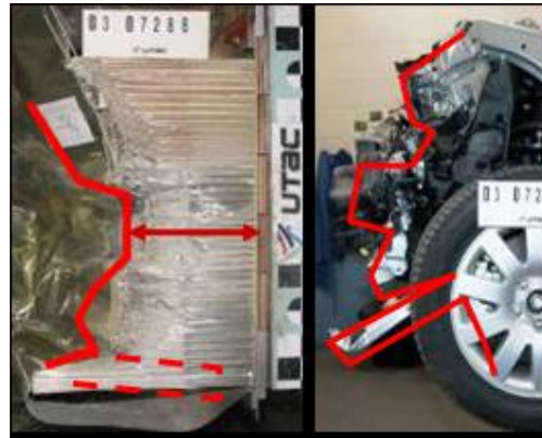
Figure 43: front deformation of the same family vehicle against PDB barrier
