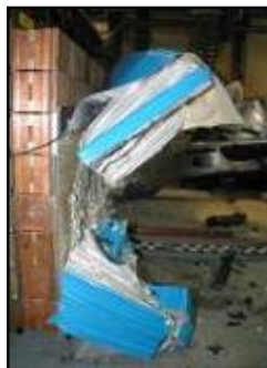
Figure 12: Current ODB barrier instability.
