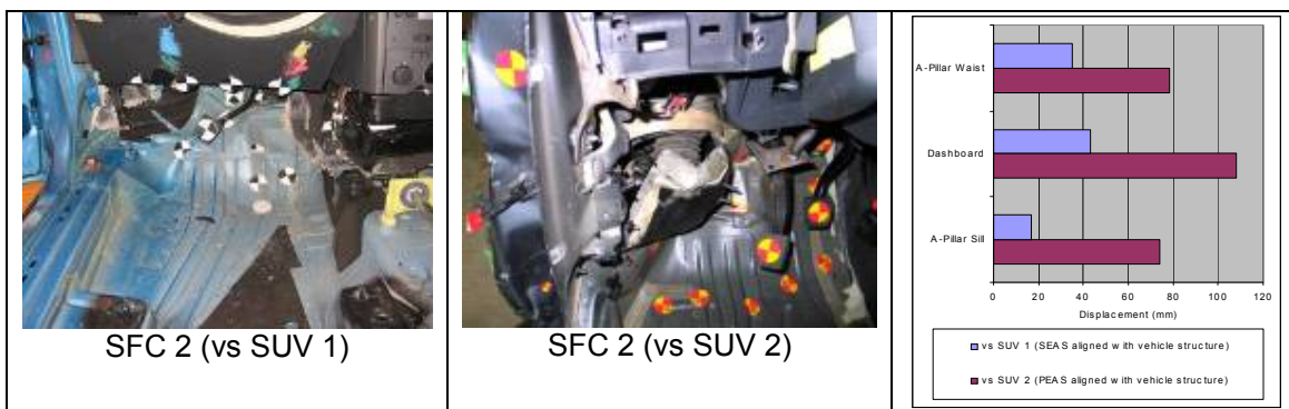
Figure 39: Deformation of the SFC 2 occupant compartment in the tests with the two SUVs (SFC 2 – SUV 1; SFC 2 – SUV 2)
