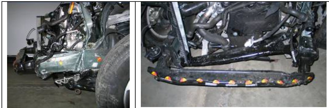
Figure 38: Deformation of the impact side lower rail and bumper crossbeam for SUV 2
