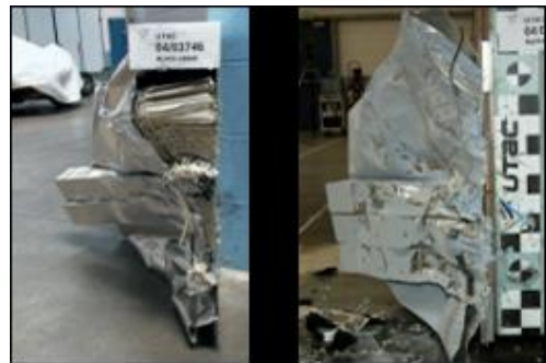
Figure 13: ODB barrier bottoming out
