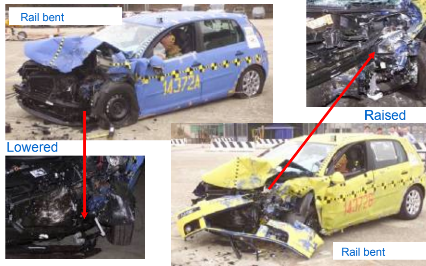
Figure 26: Car-to-car test with the single load path level SFC 3, showing the over/underriding.
