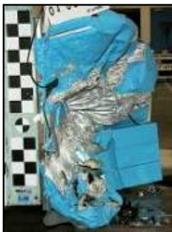
Figure 12: Current ODB barrier instability.
