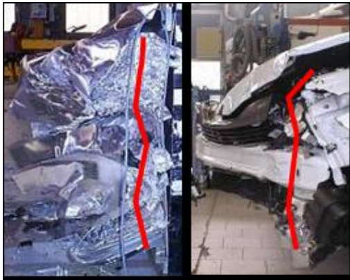
Figure 42: front deformation of 2000 kg family vehicle against current ODB barrier
