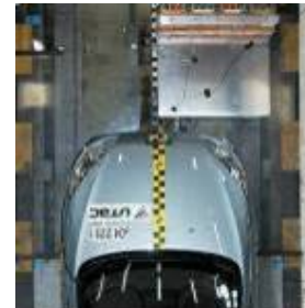
Updated ECE R94: - Test speed: 60 km/h - Overlap: 50 % - Barrier: PDB
