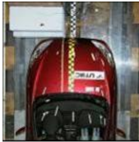
Regulation ECE R94: - Test Speed: 56 km/h - Overlap: 40 % - Barrier: current ODB
