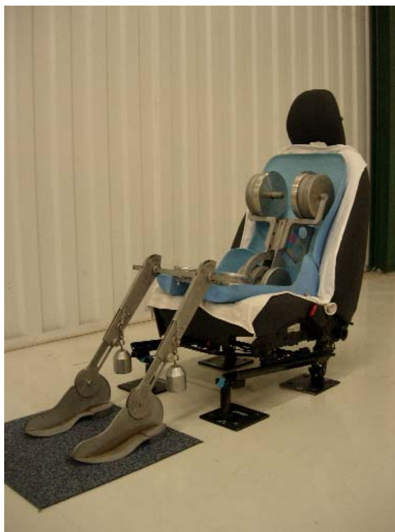
Figure A.2: 3-D H Machine manufactured by Automotive Accessories, UK
