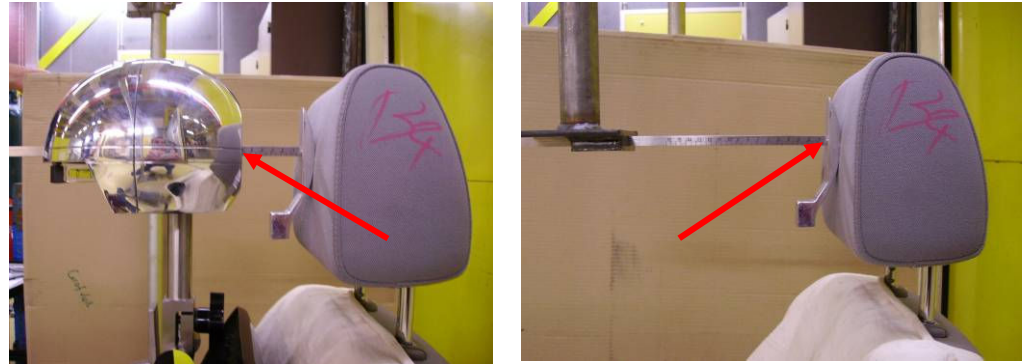
Figure 3 – HRMD measurement (left) and measurement without any seated manikin (right). Only the probe is used for backset measurement and the rear part of the HRMD head is calculated from the H-point location using fixed manikin and HRMD dimensions. The arrows indicate the CMM measuring locations.
