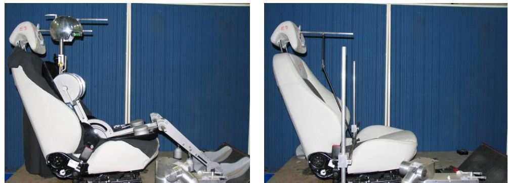
Figure 1 – HRMD backset measurement (left) and UTAC three-link bar replacement (right)
