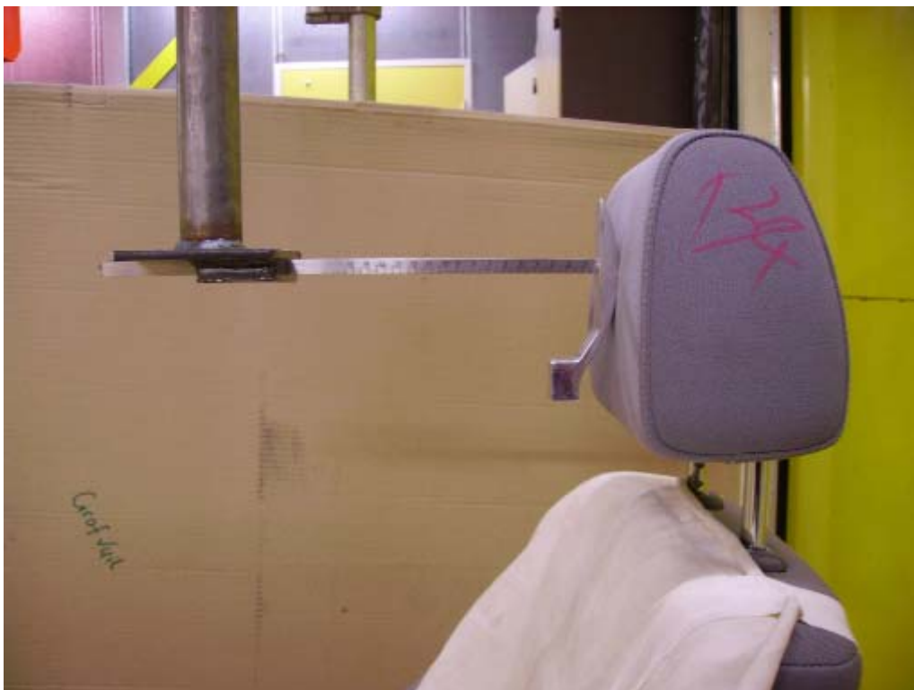
Figure 1: HRMD backset probe held in position using the adjustable portal arm
