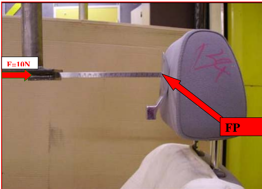
Figure 3 Measurement with the probe attached to portal in test position. The arrow indicates the FP measurement location.
