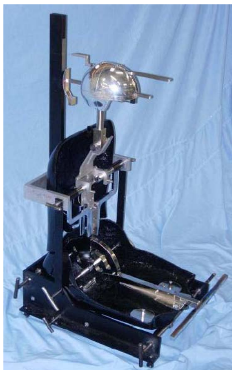
Figure A.3: The GLORIA jig for calibrating the 3-D H Machine and HRMD
