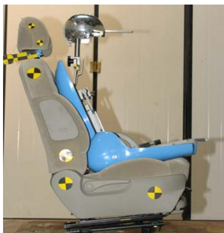
Figure C.3: 3-D H machine and HRMD
