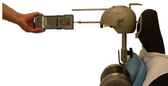
Figure C.2: Backset measurement using 3-D H machine and HRMD (EEVC WG20 method)
