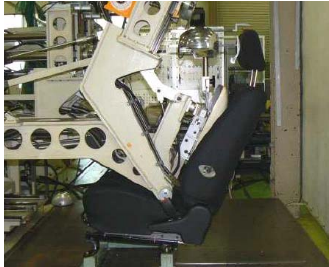
Figure C.5: OICA / JASIC approach using modified Regulation 17 equipment
