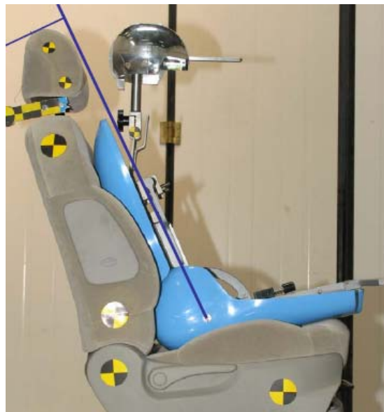
Figure B.1: UN-ECE Regulation 17 method for measuring head restraint height
