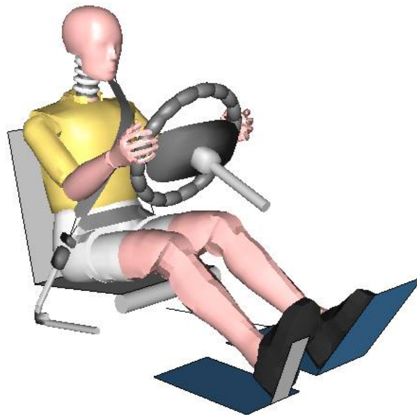
MADYMO stochastic Hybrid-III dummy model
