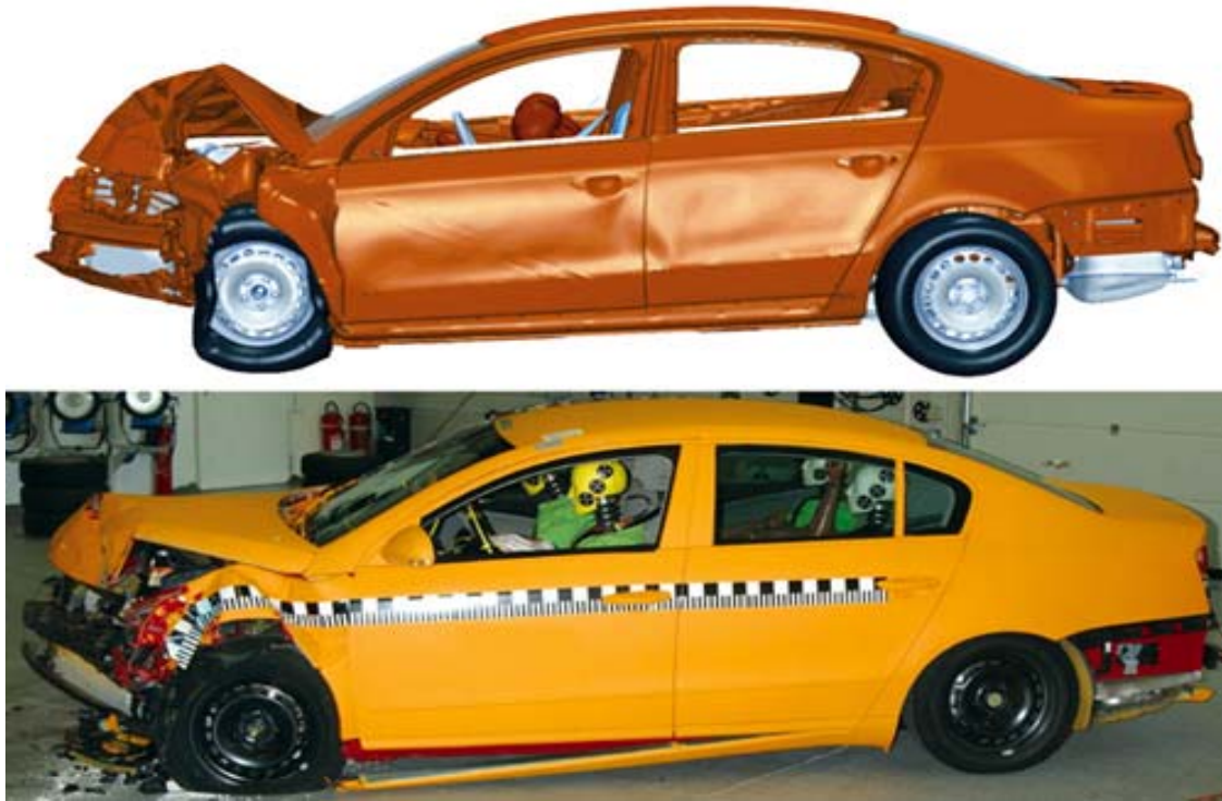
Figure 1 - Example of real and simulated frontal crash with up-to-date Finite Element simulation code ( http://www.esi-group.com/SimulationSoftware/NumericalSimulation/index_html )
