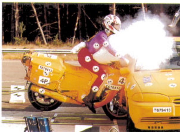
TRL: Motorcycle impact test with airbag and leg protection
