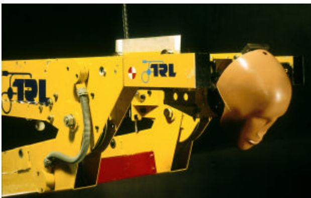
TRL: Head Protection Assessment in Side Impact
