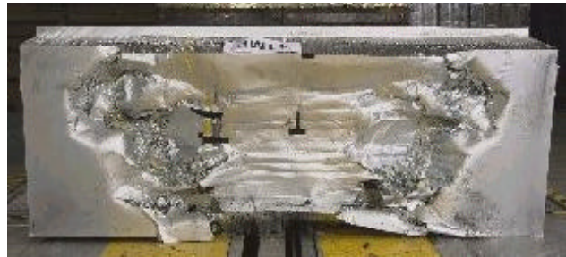
TRL : Full-Width Test against a Deformable Aluminium Honeycomb Barrier
