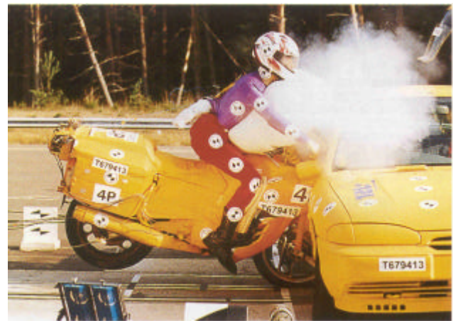
TRL: Motorcycle Impact Test with Airbag and Leg Protection
